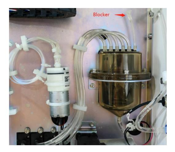
4. Check the tubes connected with RBC and WBC count chamber for dilutor. If there is much bubble in the tube, it mean that some position is leaked. We need to check the tubes and valves to confirm the problems and replace the the broken parts.
